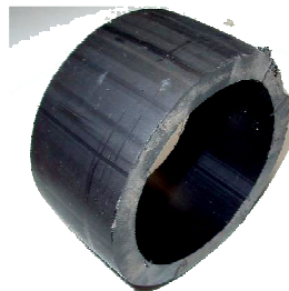
Figure 4. Example of an improper cut in pipes.
